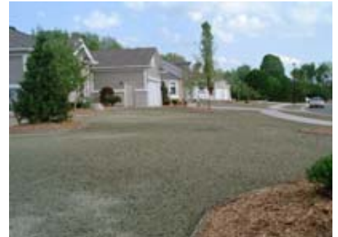
Mulch condition on mild-slope front yards after 1” rainfall
