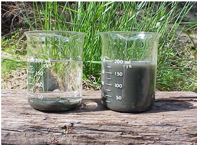
Turbid water before and after being treated with the Floc Log
