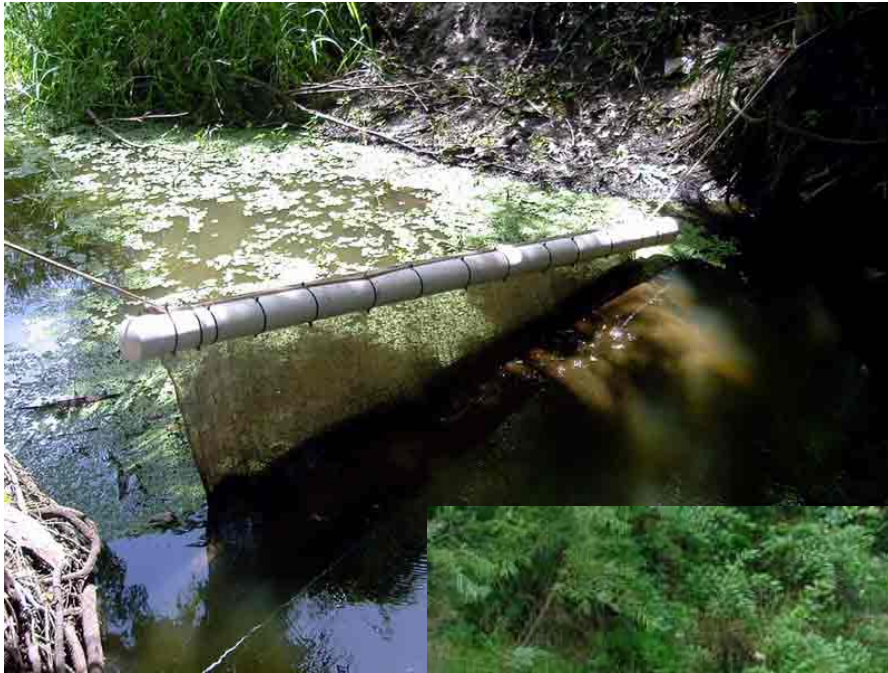
(Right) The particle curtain floating in the stream. Note the other particle curtains in place further down stream in the background.
