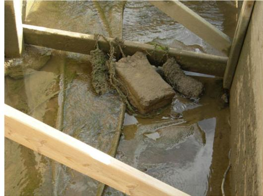
Figure 3:  $\text{CaCO}_3$  Blinding of the Floc Log
